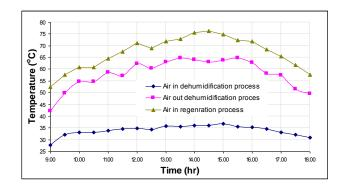
Fig.20 sensible desiccant wheel process
