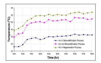
Fig.22 sensible desiccant wheel process
