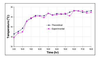
Fig.8 theoretical and experimental sensible dehumidification
