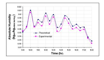
Fig.6 theoretical and experimental latent dehumidification
