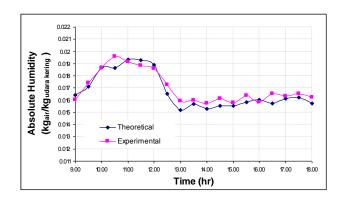
Fig.10 theoretical and experimental latent dehumidification
