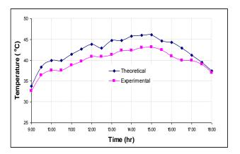
Fig.12 theoretical and experimental sensible regeneration
