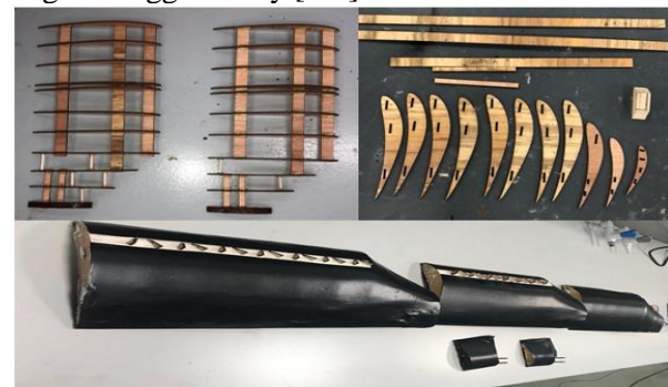
Figure 5 Wing models fabricated for Wind-Tunnel Testing.
