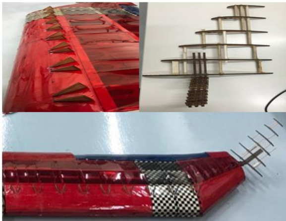
Figure 7 Final assembled wing with modifications.
