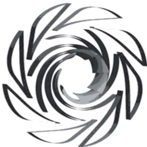
Fig.3 The SHF impeller coupled with the vaned diffuser.
