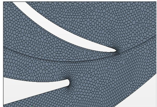
Fig.11 Local mesh between Impeller and diffuser
