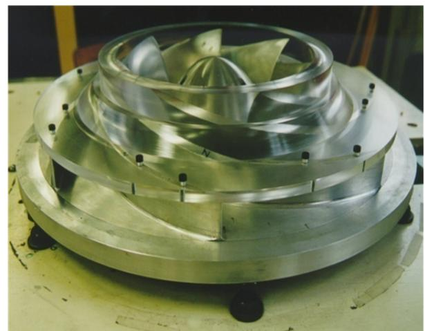
Fig.2 SHF Impeller with transparent
