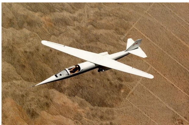
Fig 33. NASA AD-1 oblique-wing aircraft
