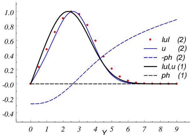
Fig. 4 Distributions of maximum,  $|u|$ , and actual,  $u$ , values of velocity perturbations and a phase shift on a boundary layer at  $Re = 200(1)$  and  $10^3(2)$  ( $M=0.2, \beta = 7 \cdot 10^{-4}$ ).
