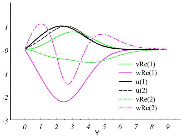
Fig. 3 Distributions of longitudinal, normal and lateral velocities perturbations and a phase shift on a boundary layer at Reynolds numbers  $200(1)$  и  $10^3(2)$ ,  $(M=0.2, \beta = 7 \cdot 10^{-4})$ .
