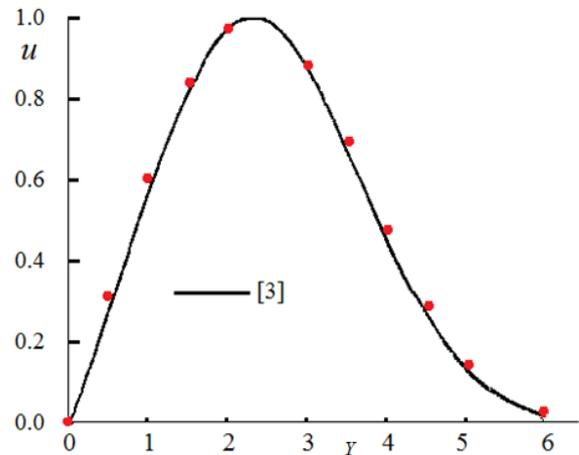
Fig. 1 Comparison of calculation results ( $M=0.2$ ) of the longitudinal velocity distribution with data of [3] ( $M=0$ ).
