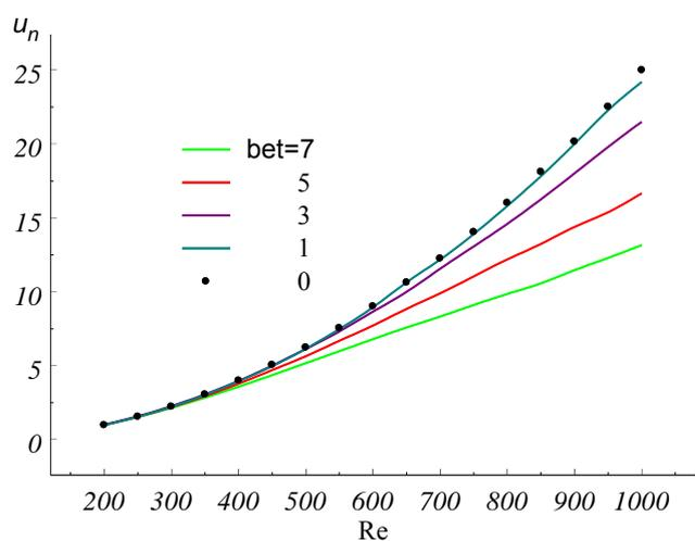
Fig. 8. Dependences of velocity perturbations amplitudes on the Reynolds number at  $M=0.2$  and different values  $bet = \beta \cdot 10^4$ .
