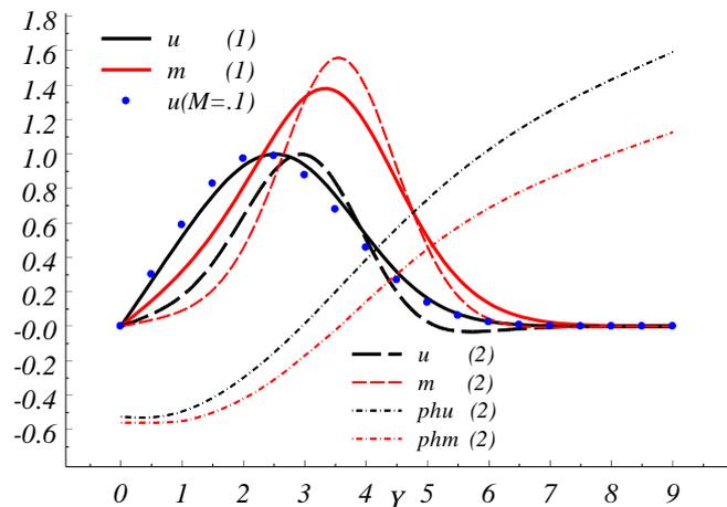
Fig. 5 Distributions  $u, m$  и  $ph$  on a boundary layer at  $M=2, Re=200(1), 10^3(2); \beta = 7 \cdot 10^{-4}$
