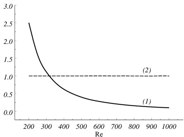
Fig. 2 Dependence of a rate amplification  $\alpha_i$  (1) and  $\lambda_1 = \alpha_i Re^2$  (2) on a Reynolds number,  $M=0.2$ .
