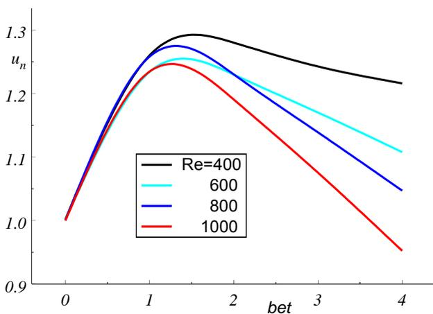
Рис. 9. Dependences of velocity perturbations amplitudes on wave number at  $M=0.2$  and different values  $Re$ .
