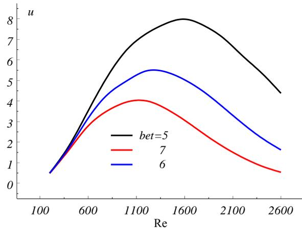
Fig. 10 Dependences of velocity perturbations amplitudes,  $u$ , on the Reynolds number at  $M=0.2$  and different values  $bet$ .
