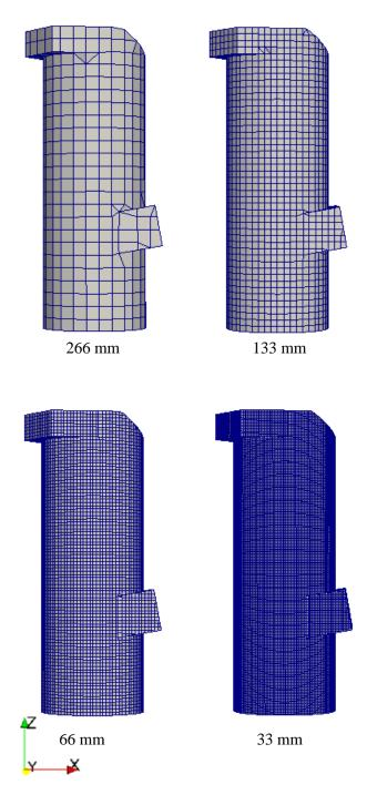
**Fig. 9** – Computational meshes labeled by different element size
