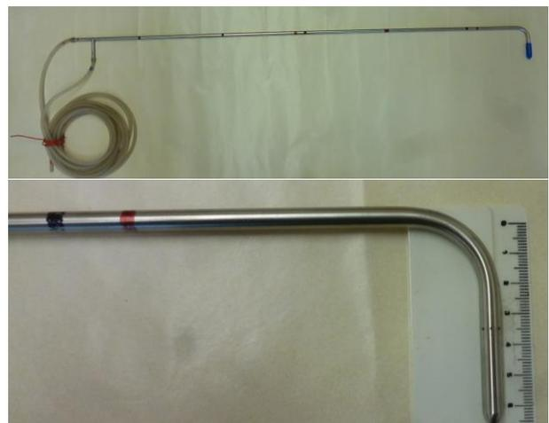
Fig. 7 – Prandtl probe with hoses and detail of measuring part
