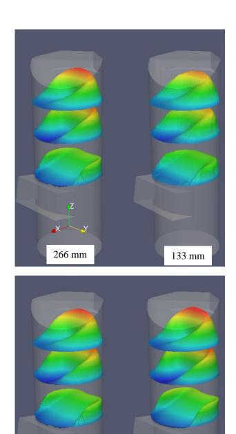
Fig. 12 – Velocity fields (CFD) – regime 40% z-velocity (m/s) for meshes with different element size
