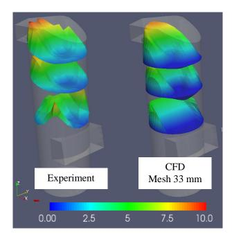
**Fig. 14** – Velocity (comparison) – regime 70%, z-velocity (m/s)
