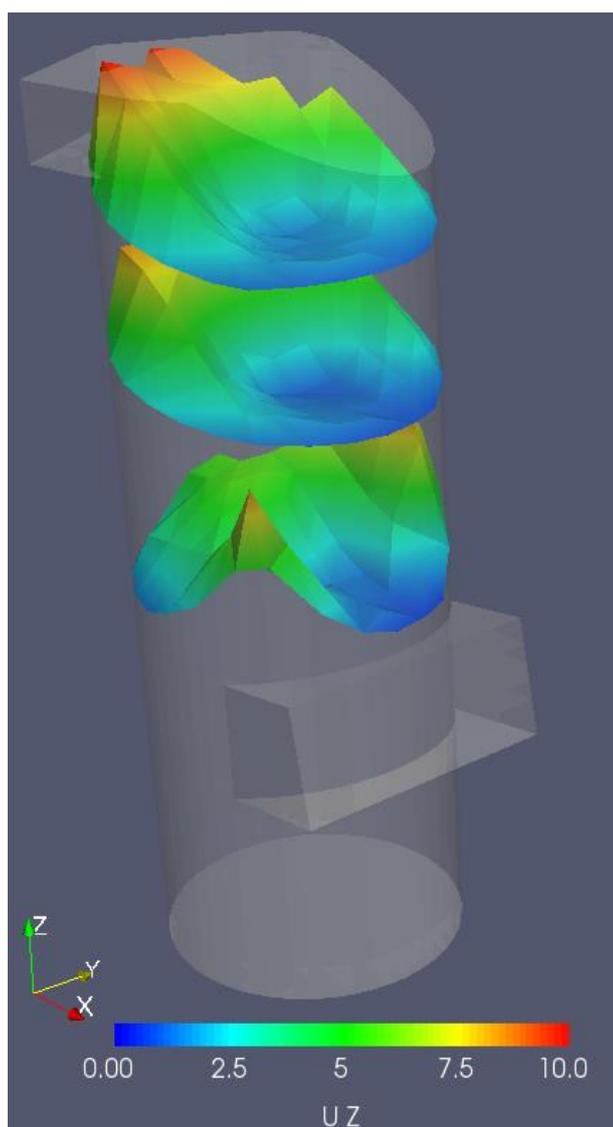
**Fig. 11** – Velocity field (exp.) – regime 70% z-velocity (m/s)
