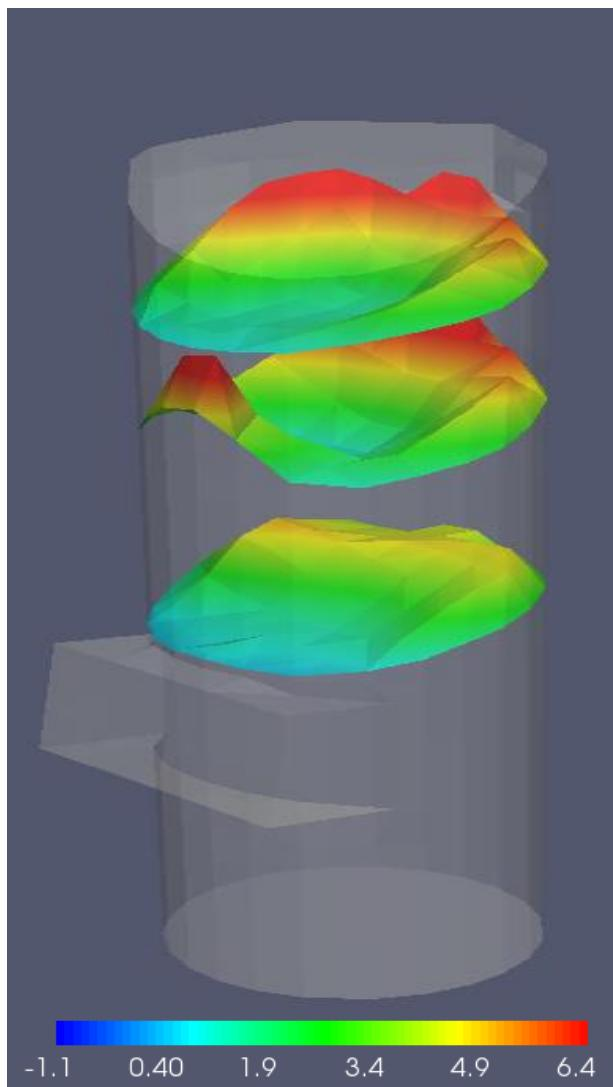
**Fig. 10** – Velocity field (exp.) – regime 40% z-velocity (m/s)
