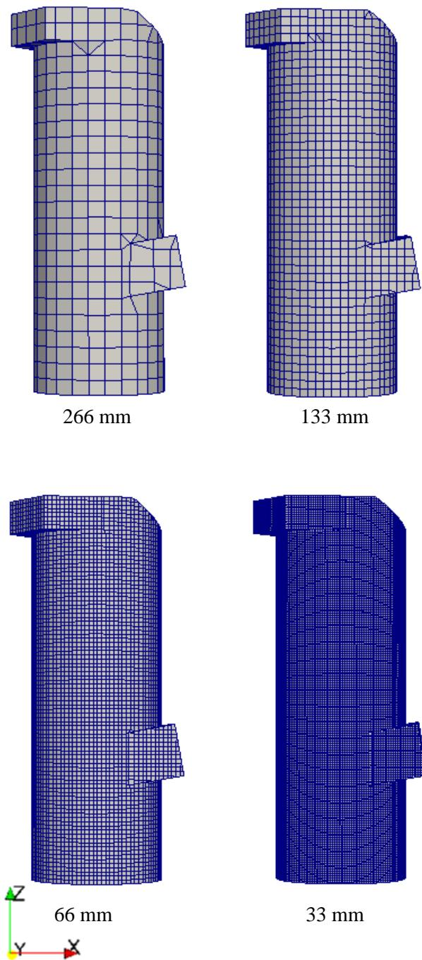
**Fig. 9** – Computational meshes labeled by different element size
