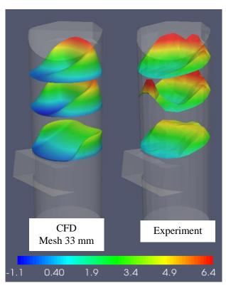
**Fig. 13** – Velocity (comparison) – regime 40%, z-velocity (m/s)
