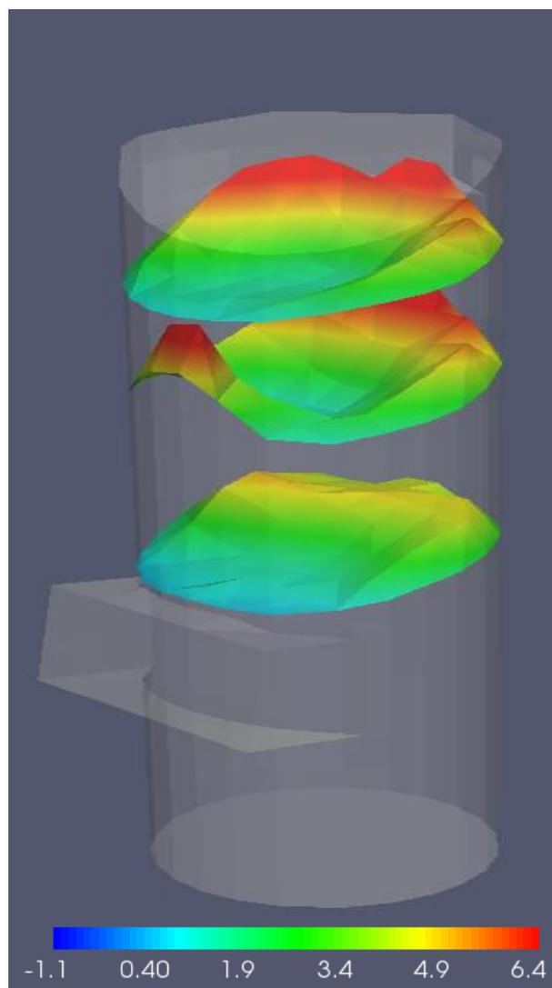
**Fig. 10** – Velocity field (exp.) – regime 40% z-velocity (m/s)
