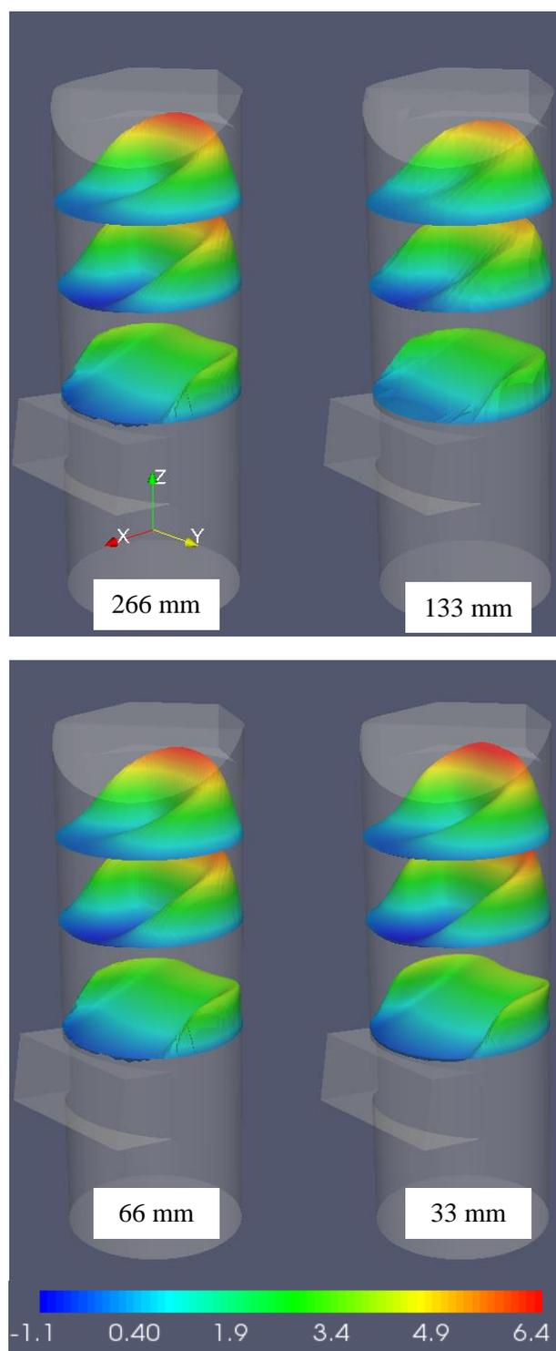
**Fig. 12** – Velocity fields (CFD) – regime 40% z-velocity (m/s) for meshes with different element size
