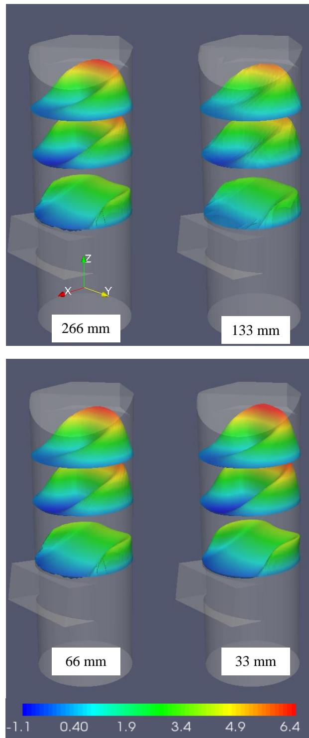
**Fig. 12** – Velocity fields (CFD) – regime 40% z-velocity (m/s) for meshes with different element size
