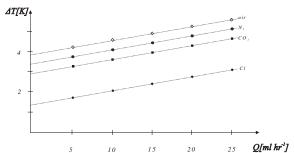
Figure 6: The functionality  $\Delta T$  on flow rate Q at downstream sensor  $R_R$ , constructive material steel
