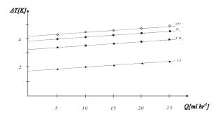
Figure 8: The functionality  $\Delta T$  on flow rate Q at upstream sensor  $R_U$ , constructive material plexi – glass
