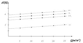
Figure 9: The functionality  $\Delta T$  on flow rate Q at upstream sensor  $R_U$ , constructive material steel
