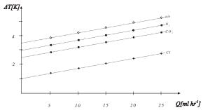
Figure 7: The functionality  $\Delta T$  on flow rate Q at downstream sensor  $R_D$ , constructive material cooper
