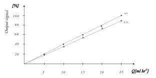
Figure 17: Measurement results obtained with gas flow sensor (downstream sensor) with flow range 25  $ml/h \equiv 100 \%$  according to the time – of - flight measurement principle and its working range; the flow tube is made of stainless steel and have an internal diameter of 1 mm.
