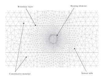
Figure 3: Partial view of the computational grid for the basic configuration
