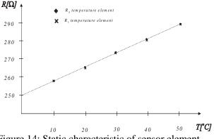
Figure 14: Static characteristic of sensor element
