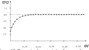
Figure 15: Dynamic characteristic of sensor element
