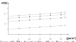
Figure 10: The functionality  $\Delta T$  on flow rate Q at upstream sensor  $R_U$ , constructive material cooper
