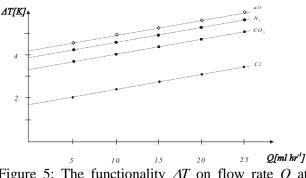
Figure 5: The functionality  $\Delta T$  on flow rate Q at downstream sensor  $R_D$ , constructive material plexi – glass
