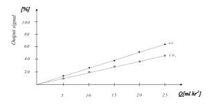
Figure 18: Measurement results obtained with gas flow sensor (upstream sensor) with flow range 25  $ml/h \equiv 100$  % according to the time – of - flight measurement principle and its working range; the flow tube is made of stainless steel and have an internal diameter of 1 mm.
