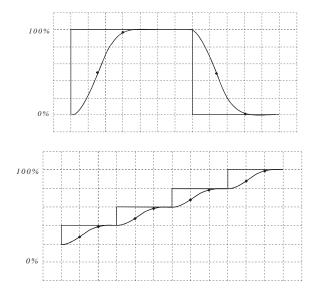
Figure 19: Measured response times of a gas flow sensor adjusted for air:  $25 \ ml/h \equiv 5 \ V$ ; the X - axis
