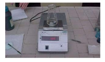
Fig. 2. Solute concentration of CMC-water solutions is set by using precision scale and a 250-ml flask. Kinematics can be therefore described by processing them with a PIV technique. Dynamics can be described as well, by measuring wall stresses [36] by specific sensor probes.
