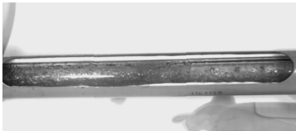
Fig. 13. Snapshot of the oil air mixture flow in the horizontal pipe section
