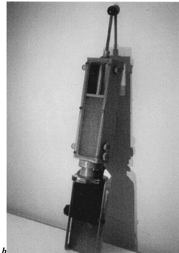
Fig. 5. Experimental cells used for capillary driven seepage flows studies under variable gravity conditions.
