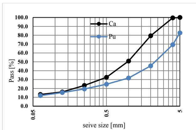
Fig.1. Grading curves of calcareous and pumice sand.
