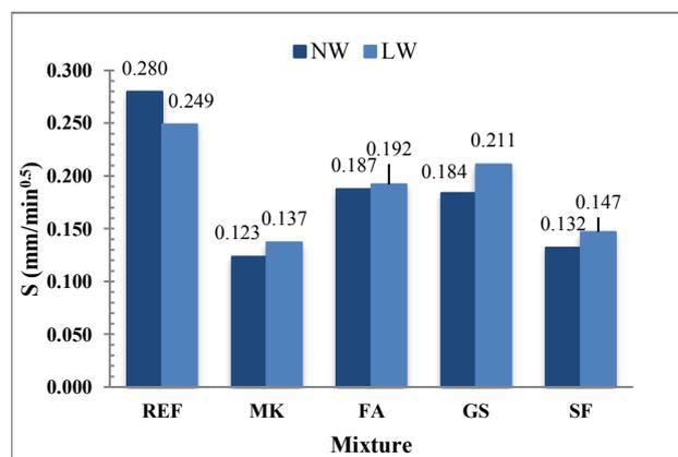
Fig.3. Sorptivity of NW and LW mortars, for samples aged 28 days.
