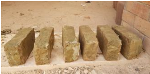
Fig. 5. Moulds removed, bricks left to air-dry
