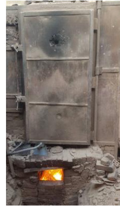
Fig. 6. Oven-kiln firing the bricks
