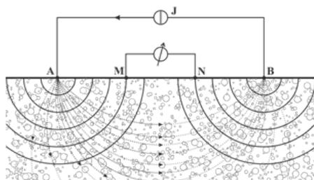
Fig. 1: The arrangement of the electrodes, an image of the current lines and surface potentials in homogenous, isotropic sub-soil with an AMNB, Schlumberger array [6]
