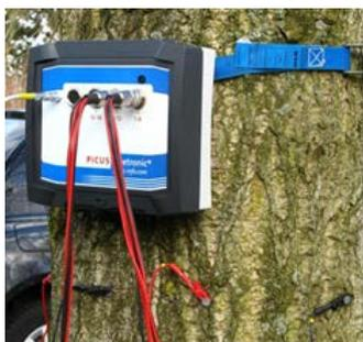
Fig. 2: The PICUS Treetric measuring system [16]
