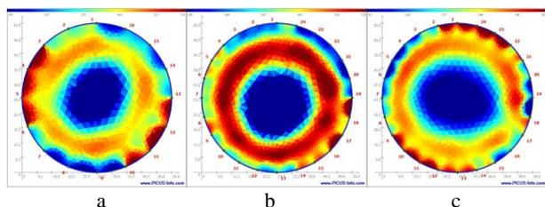
Fig. 6: EIT tomograms of measurements performed on old common oaks ( $\Omega\text{m}$ )
