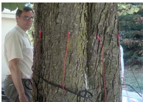
Fig. 3: Installing electrodes to a tree trunk at chest level
