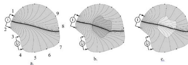
Fig. 4: The principle of EIT in assessing living trees (a. homogenous distribution of conductivity b. and c. examples for inhomogeneous distribution of conductivity) [16]
