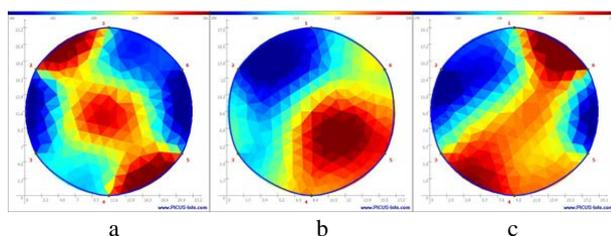
Fig. 5: The EIT measurement results performed on middle-aged Austrian oaks ( $\Omega\text{m}$ )
