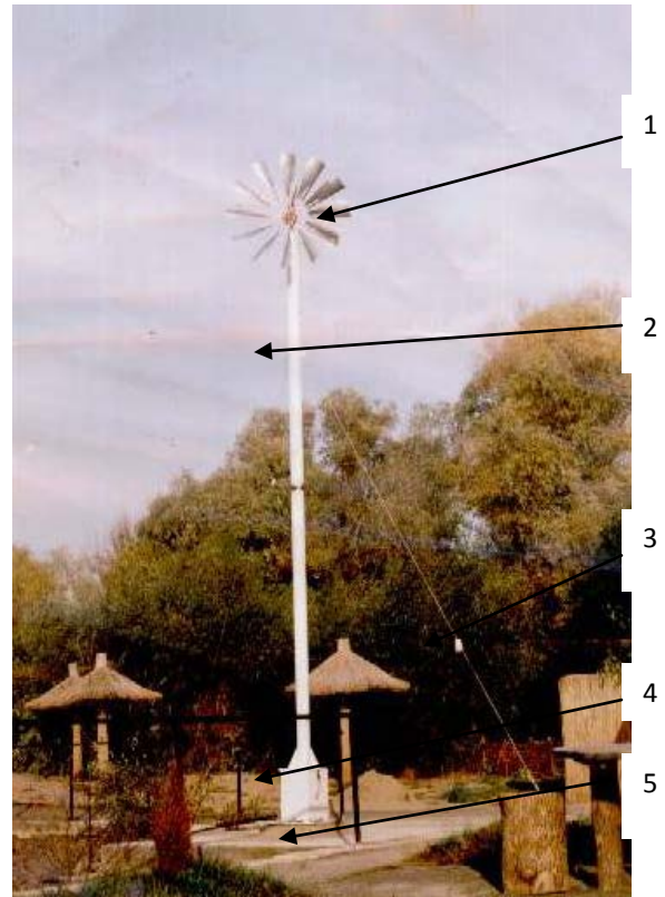
Fig.1: A wind turbine with horizontal axis to pump water.
