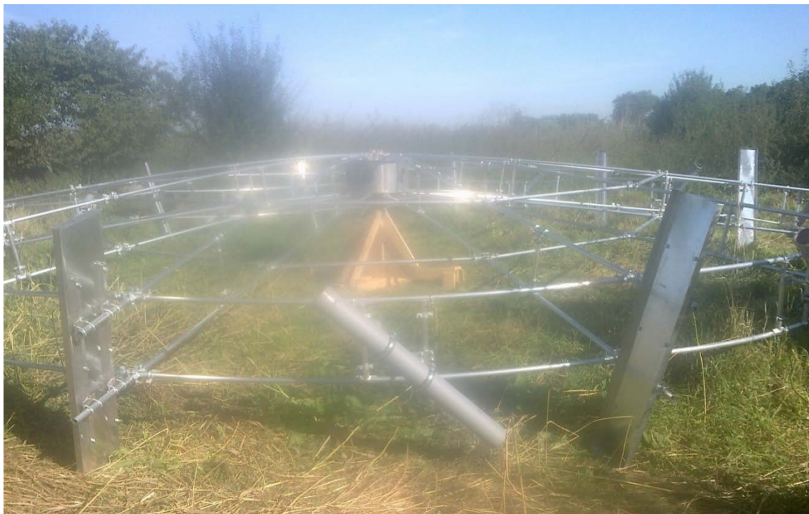
Fig.9: Rotor of a water wheel with a diameter of 10 m.
