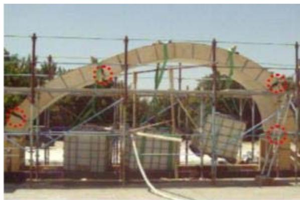
Fig. 7. Collapse mechanism and achievement of the hinges in the arch with an asymmetric load condition.
