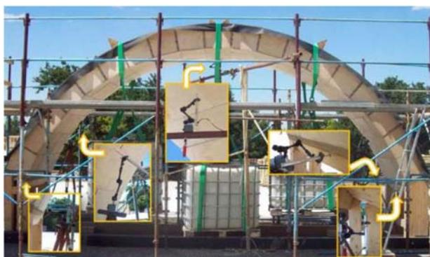
Fig. 6. Tested arch with details of the positioning of the displacement transducers.
