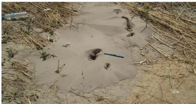
**Figure 7:** Kato Achaia-East: Sand craters with the emergence of the liquefied soil of silt composition [Source: ITSAK, 2008 [23]- Batilas, Athanasopoulos, Pelekis P, Vlachakis, Klimis, Mylonakis (2010) [21]]
