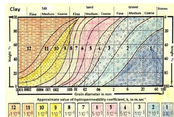
**Figure 4:** Typical values of the permeability coefficient  $k$  for various soil formations [Source: Poursaitidis, 2013] [7]
