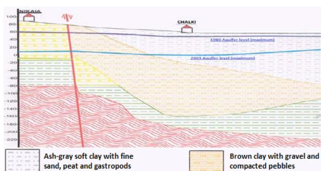
**Figure 16:** Soil profile and fall of the water surface in the area of Halki [Source: Hatzopoulou, 2018 [26], Dakoulas, Thanopoulos, Belesis, Lazaropoulos, 2004 [27]]
