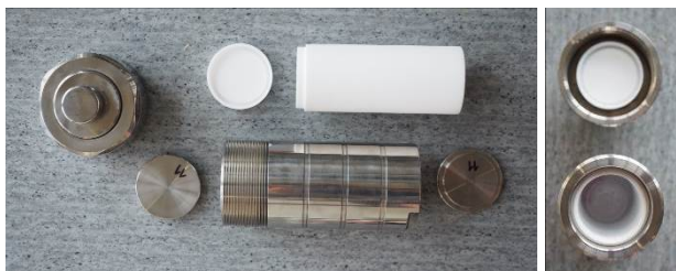
Fig. 4. Used autoclave reactor (250 ml), components (left), before inserting a sample and closing (right)
