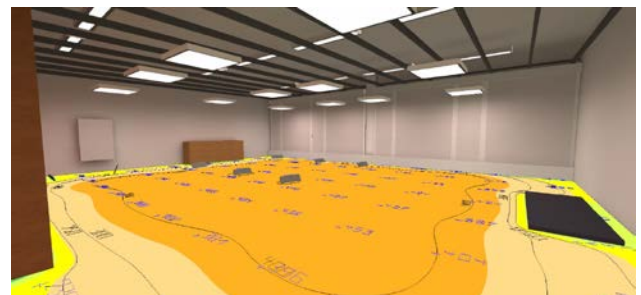
Fig. 9. Example of the illuminance distribution on a work plane throughout the lab.
