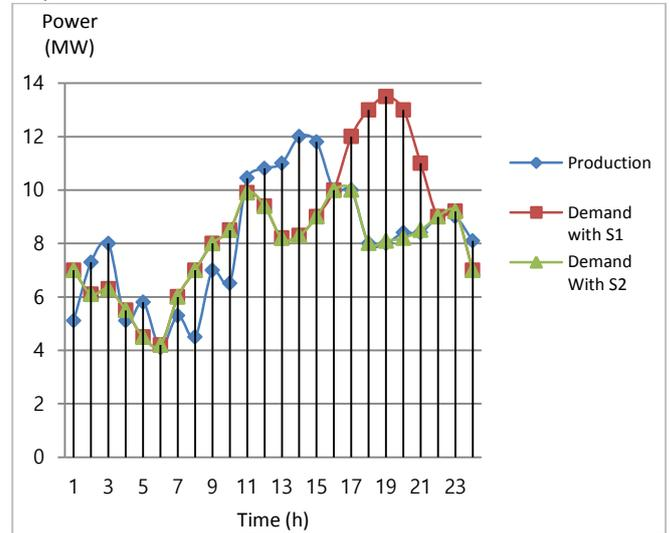
**Fig 6.** Real-time illustration of demand reductions during peak hours of scenario (S2).
