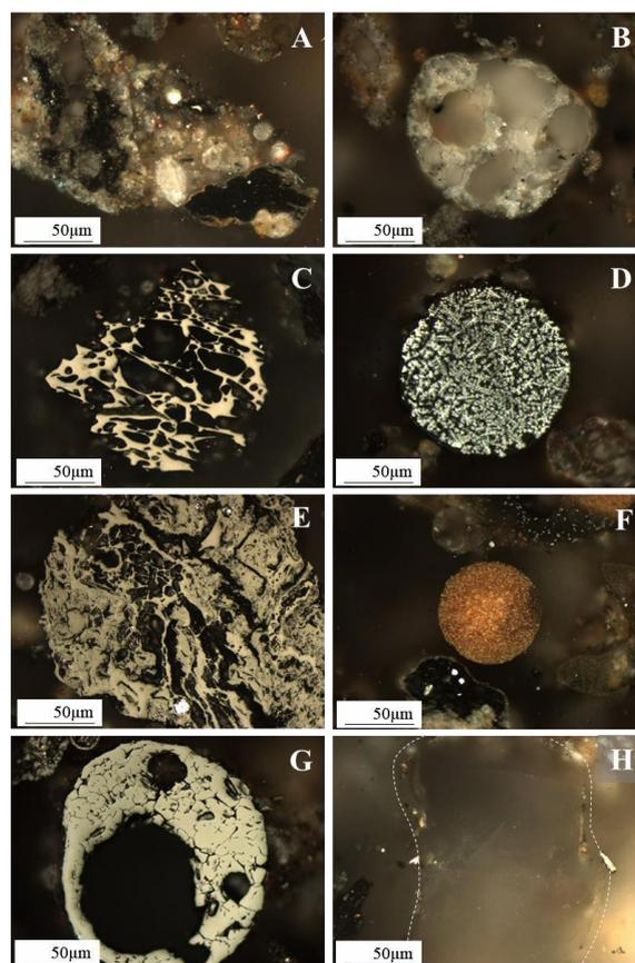
Fig. 3 Bottom ash morphotypes (reflected white light, + polars;  $\times 500$ ) A) partially baked clay (sample MS1; + polars); B) glass (sample MS3); C) char (sample MS5); D) ferrosphere (MS1); E) oxidized Fe (sample MS2); F) calcisphere (sample MS1); G) magnesiassphere (sample MS1); H) quartz (dashed lines limiting; sample MS5).
