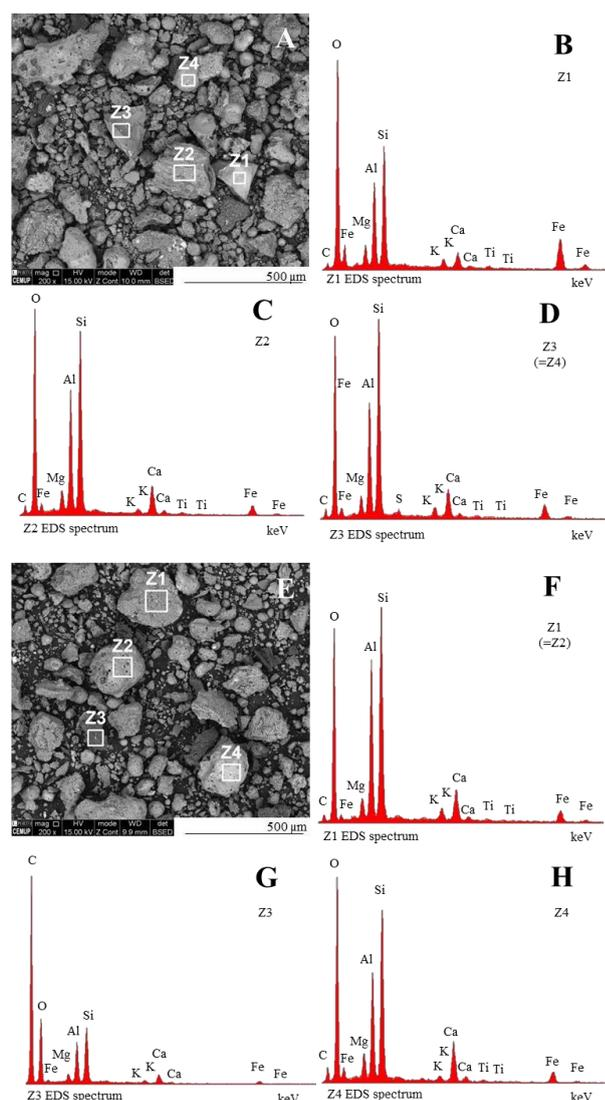
Fig. 6 SEM/EDS analysis of the bottom ash (backscattered electron mode): A to D) fraction separated using a Nd hand magnet (Sample MS2); E to H) fraction separated using Stearns magnetic separator at 10500 Gauss (Sample MS3).
