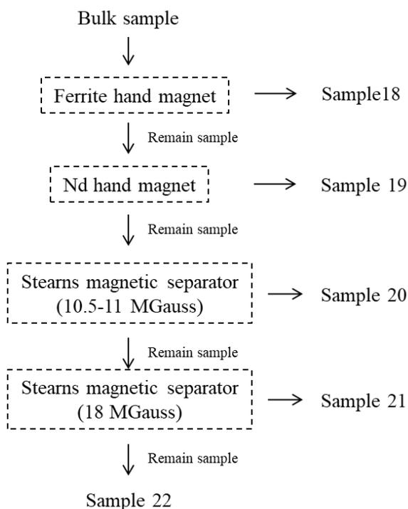
Fig. 2 Magnetic separation scheme.
