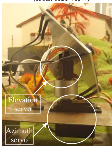
Figure 25: small scale solar tracking system (back side view)
