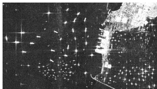
Fig. 1 One Sentinel-1A SAR image of the study area, at the Johor Strait. The goal is to detect the large vessels that offer no reasonable doubt, discarding speckle effects ("stars") and small fishing boats, and discriminate between large and very large ships.
