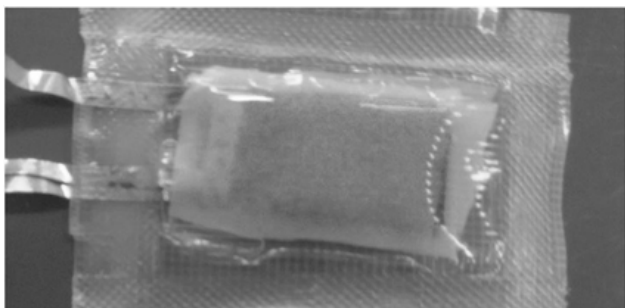
Fig.7. A model Ni-MH cell of pouch type with PVA/AG/50%KOH electrolyte.
