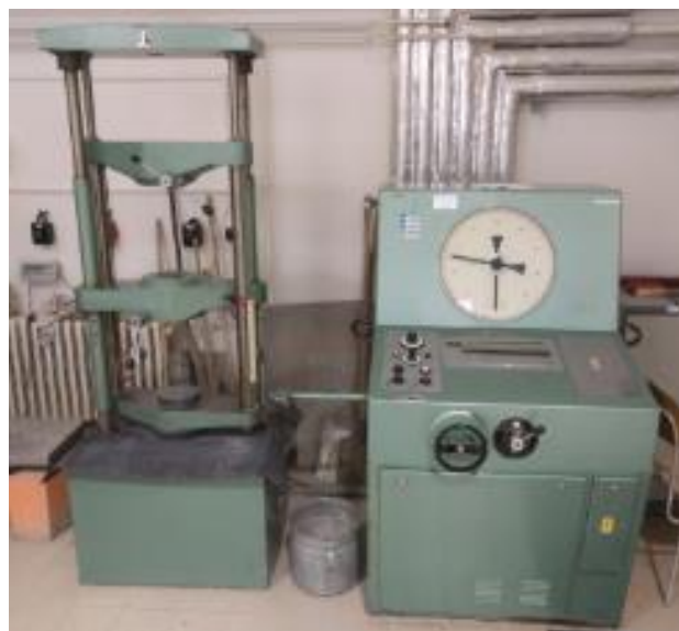
Fig. 7 device for determination of compressive and tensile strength
