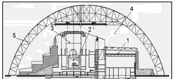
Fig. 5. The scheme of the SO and the NSC cross-section. 1- turbine hall, 2 – destroyed reactor, 3 – central hall, 4 – main volume and 5 – annular space of the NSC.
