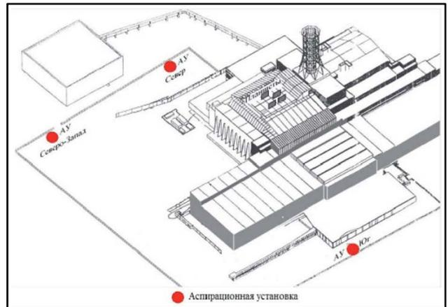
Fig. 14. The Aspiration Units and accumulating pads location scheme nearby the SO and the SO roof.
