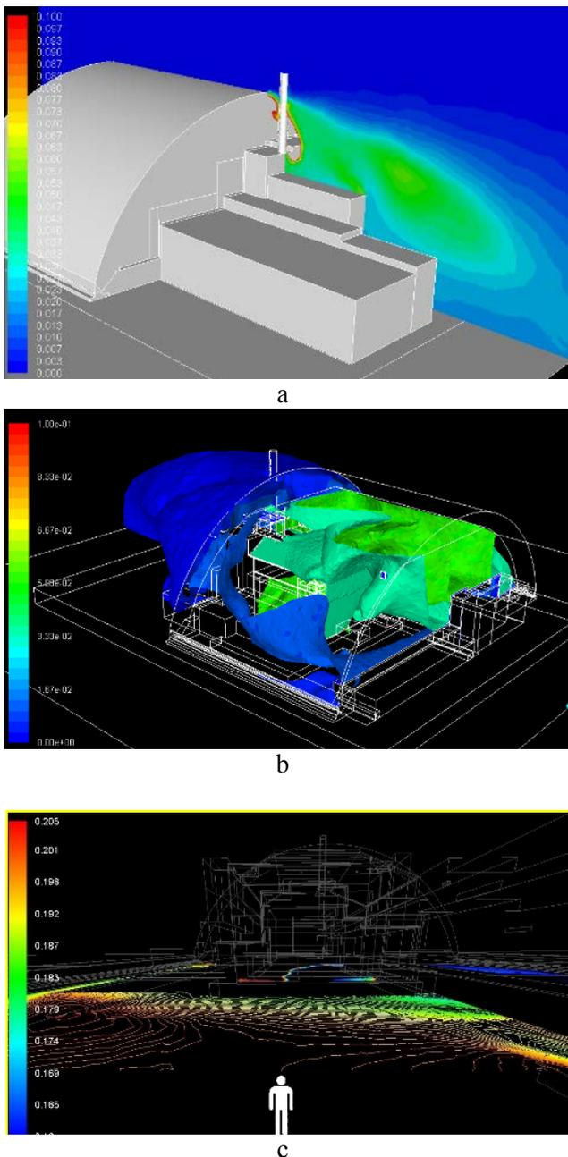
Fig. 19. RA concentration distribution,  $Bq/m^3$ , (a) outgoing from NSC to the environment, (b) isosurfaces of RA concentrations inside and outside the NSC, and also (c) isolines of RA concentrations inside the NSC at the height of 1.5m from the ground at the area of possible personnel activity.
