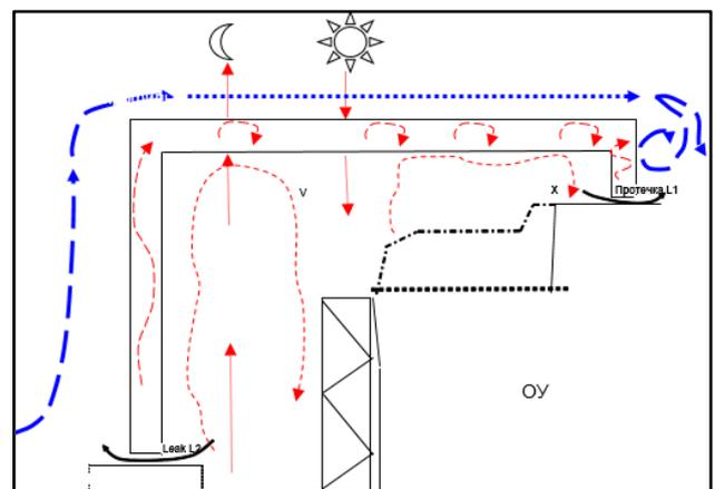
Fig.9. Longitudinal section of NSC and SO. The blue arrows on indicate the outside airflow movement due to wind and pressure difference and the red arrows inside due to thermally induced airflow movement due to temperature differences (thermal convection).
