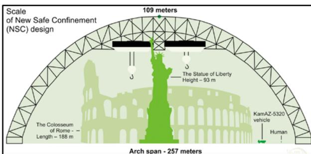
Fig. 8. Comparative sizes of the New Safe Confinement
