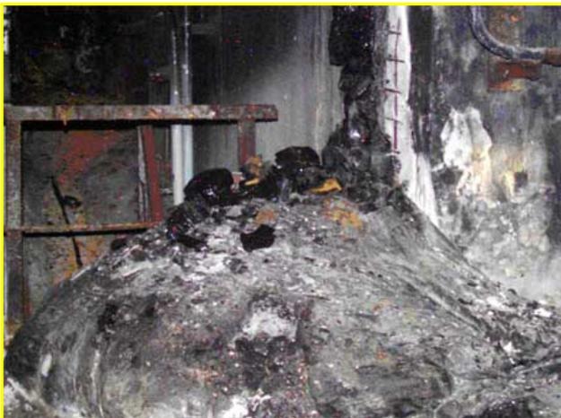
Fig.3. Highly radioactive melted fuel masses under destroyed reactor in the Shelter Object (Fig. 2, red zones).
