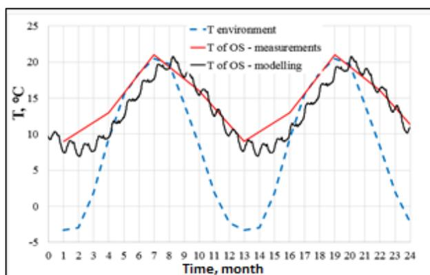
Fig. 16. Dynamic changes of average temperatures (T) of SO inner volumes and environment during two years
