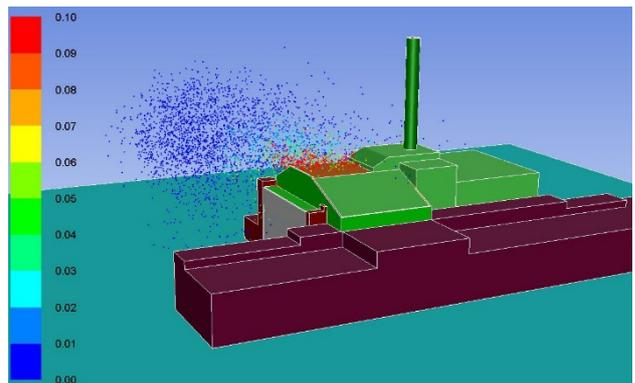
Fig. 15. Visualization of RA emissions through the SO roof of the model in the south wind.
