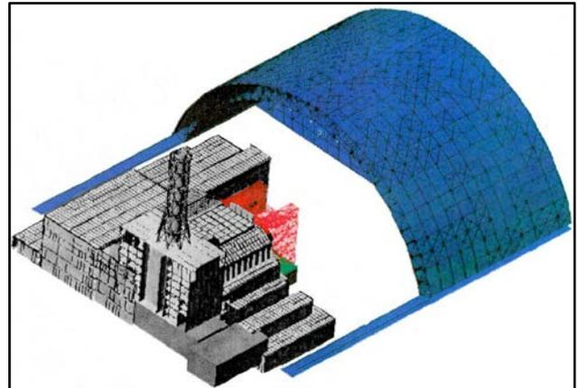
Fig. 4. The scheme of the SO and the NSC relative position.
