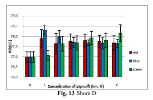
Hardness results (Shore D) show that when a red pigment was added to the PC material (Lexan 923), the hardness increased and the trend was decreasing with increasing concentrations. A similar phenomenon occurred with the use of a blue pigment. On the other hand, the green pigment showed a growing trend.
