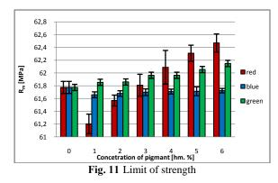
The tensile test indicates the strength of the material. When the red or green pigment was added to the natural polymer (lexan 923), the tensile
