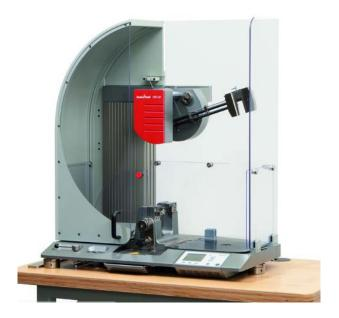
Fig. 6 Impact bending test
