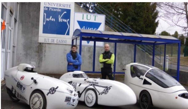
Fig. 1: Various prototypes of motorized electric cycles fully faired (50 kg to 85 kg)
