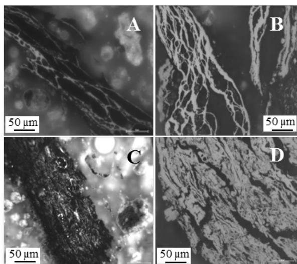
Fig. 3. Photomicrographs of carbonaceous residual carbon in Turceni (A, B, and D) and Govora (C) samples (reflected light microscopy, glycerin immersion  $\times 350$ ): A, B) degassed char particles originating in xylite cellular textinite; C) partially degassed char particle originating in huminite; D) non-degassed unburned coal particle originating in ulminite [10].
