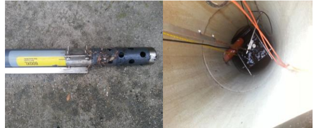
Fig. 9 the multi-parameter water sensor in the drainage shaft near the PK6 building
