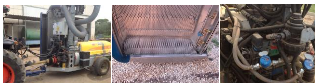
Fig. 2. Recovering system (left); recovery tray (center); hydroinjectors, return lines, filters (right), the inserted flowmeters during the tests are shown.
