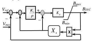
Fig.12 . Regulating scheme for the effective value  $(V_{mes})$  of the inter-phase network voltage (IP controller)
