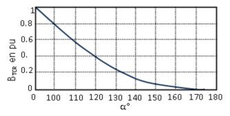
Fig. 3. Characteristic of susceptance
