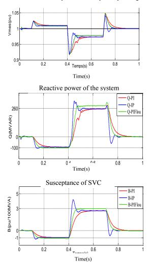
1. Measured amplitude of the primary voltage
