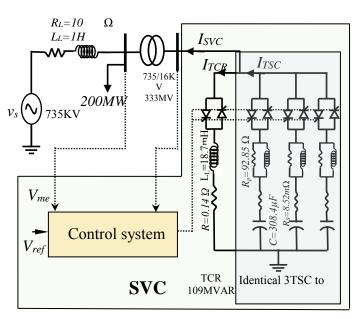
Fig.11. Overall scheme of the system to simulate (single-line diagram)
