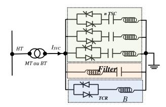
Fig. 8. General structure of an SVC
