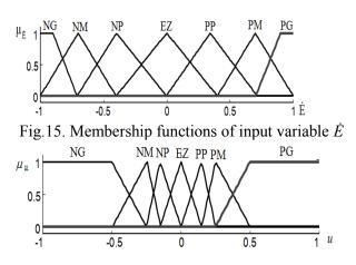
Fig.16.Membership functions of output variable u
