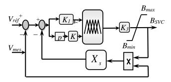
Fig. 13. Regulatory scheme of the rms value (V<sub>mes</sub>) of the inter-phase network voltage (PI Blur regulator)
