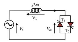
Fig.1. Single-phase circuit of a TCR
