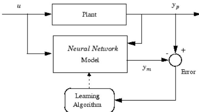
Fig.9. NNMPC System Identification
