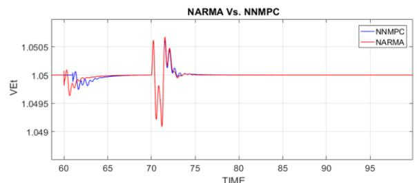
Fig.18: Terminal voltage ( $V_{Et}$ ) Real Power flow ( $P_2$ ) in case of sudden system disturbance
