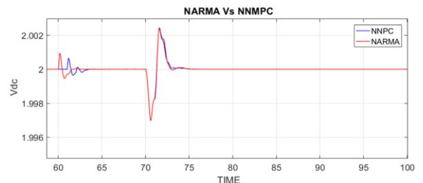
Fig.17: DC line voltage ( $V_{dc}$ ) in case of sudden system disturbance
