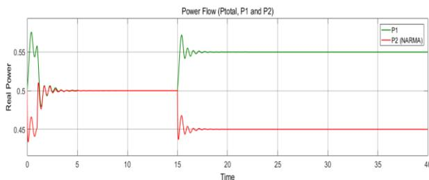
Fig.14. Real Power flow in line 1 and 2 by using NARMA-L2 in case of sudden step change (-10%)
