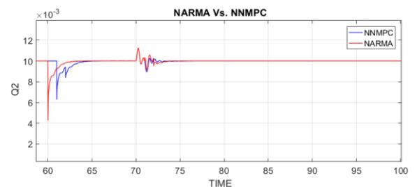
Fig.16: Reactive Power flow ( $Q_2$ ) in case of sudden system disturbance
