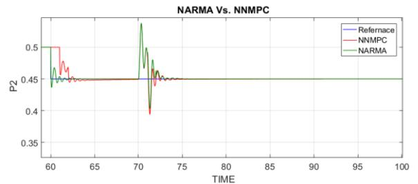
Fig.15: Real Power flow ( $P_2$ ) in case of sudden system disturbance
