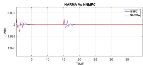
Fig.12: Dc Line Voltage ( $V_{dc}$ ) in case of sudden step change (-10%)
