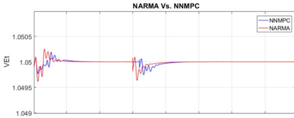
Fig.13: Terminal Voltage ( $V_{Et}$ ) in case of sudden step change (-10%)
