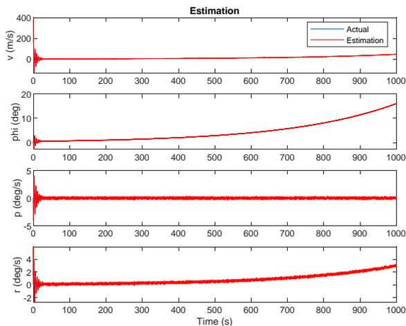
Fig.3. Estimation results of the lateral motion parameters: actual value-blue line; estimated value-red line.
