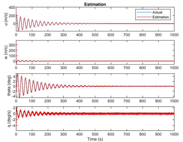
Fig.2. Estimation results of the longitudinal motion parameters: actual value-blue line; estimated value- red line.
