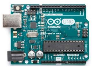
Fig. 6. Arduino Uno microcontroller [16]
