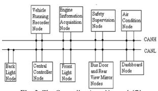
Fig. 3. The Controller Area Network [7]
