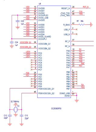
Fig. 3 The node design does not directly use 2538 USB function instead of using the PL2030 USB
