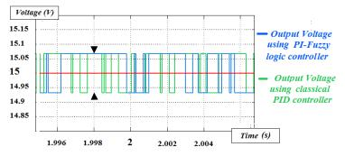
Fig.10 Output voltage ripple.
