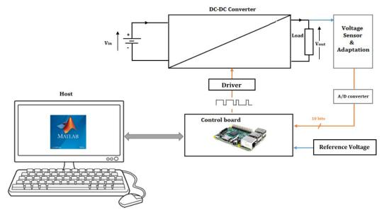
Fig.1 The proposed block diagram system.
