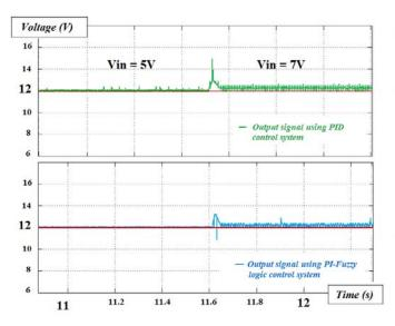
Fig.7 Simulation with irregular supply voltage.
