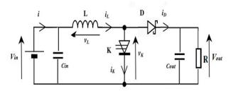
Fig.2 Topology of the Boost converter.
