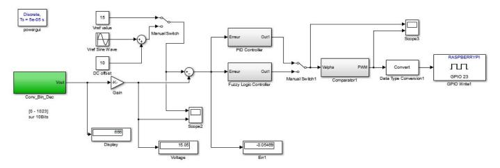
Fig.4 Block diagram of the implemented control system.
