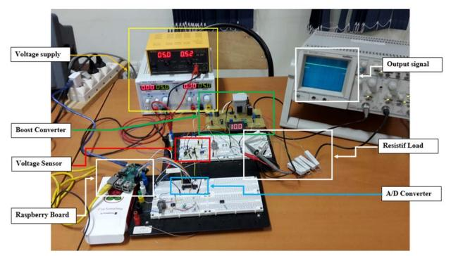
Fig.6 The experimental hardware setup.
