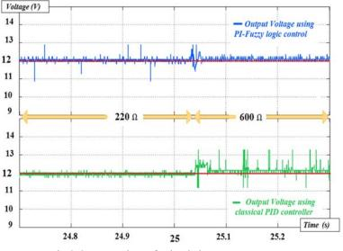
Fig.8 Output voltage for load change case.
