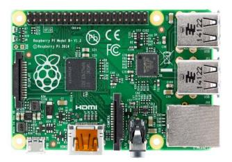
Fig.3 Raspberry Pi 2 B 32-bit microcontroller board
