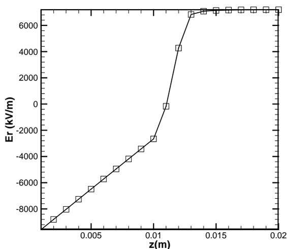
**Fig. 10 Space charge field distribution at  $t=2.22$ ns and  $P=100$  torr under  $E_0=7000$  kV/m**
