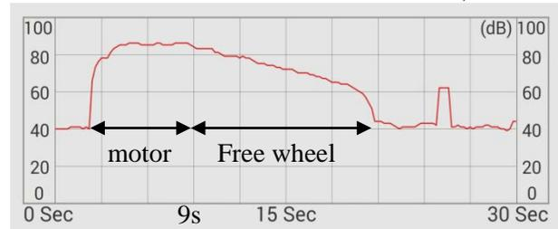
fig 19: Noise wheel electric motor to 30 cm
