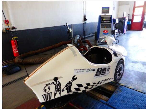
fig 17: Roadworthiness testing of brakes and shock absorbers
