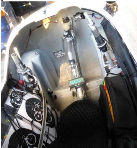
fig 18: Handlebar (inside the electric Velomobile Leiba XStream) [5]
