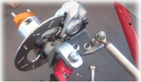
Fig. 8. Study of floating front brake by the students of Mechanical Engineering IUT of Aisne.
