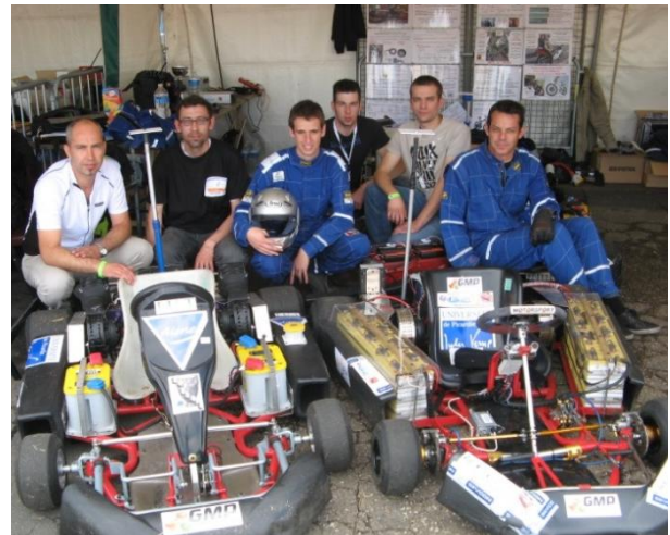
Fig. 5. Electric Go-Karts, rating motors 28 kW : 48V lead-acid batteries on the left and 72V LiFePo batteries on the right. International e-Kart Challenge in Vierzon (France) 2011.
