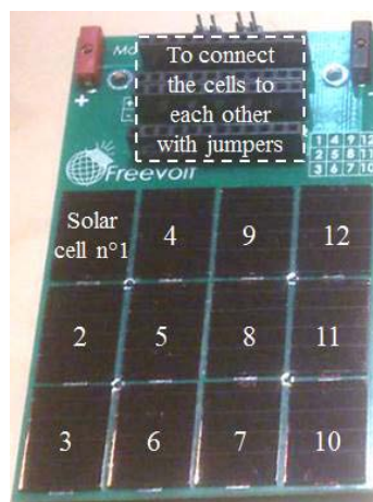
Fig. 3 – Solar matrix used to build a whole photovoltaic power system.
