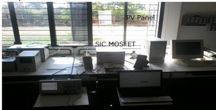
Figure.23.Hardware set-up for fuzzy MPPT control based photovoltaic power generation system
