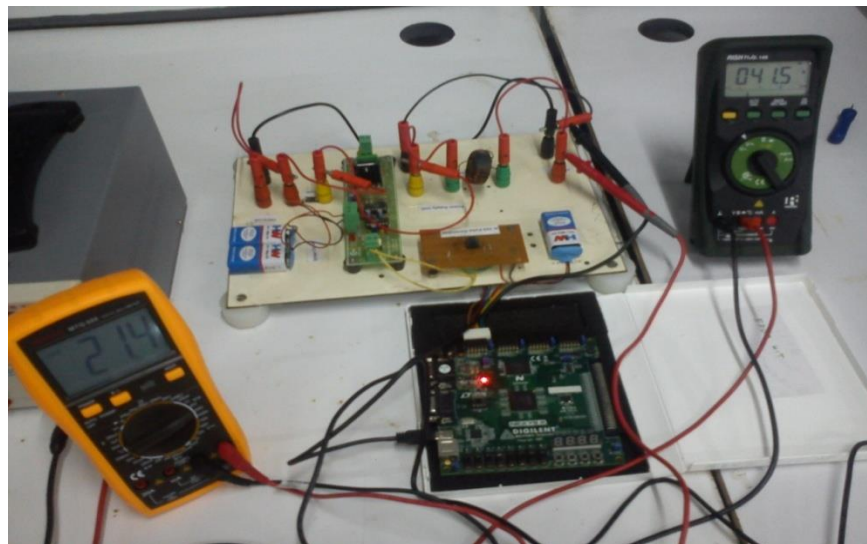
Figure.27. PWM output for 50% duty ratio
