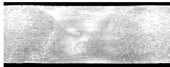
Fig. 2. The section of the joint welded by FSW method in two passages. 5083 alloy. Etching with Keller's reagent.
