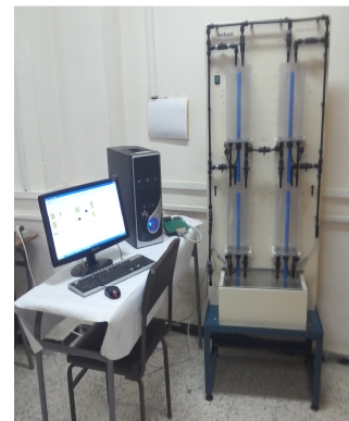
Figure 3: Coupled tank process linked to the computer
