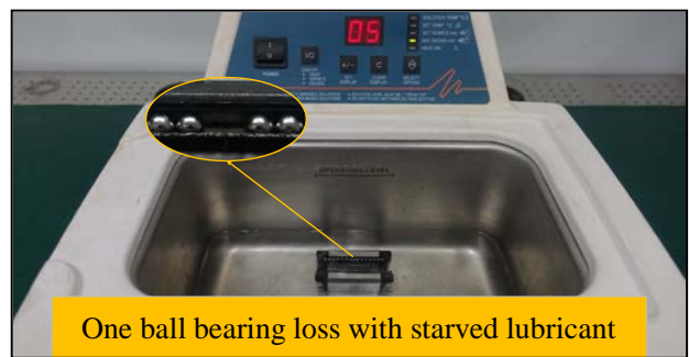
Fig.13 One ball bearing loss in ultrasonic cleaning
