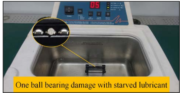
Fig.12 Ball bearing damage in ultrasonic cleaning machine
