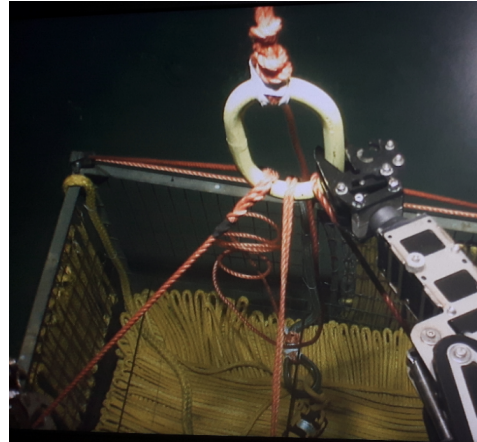
Figure 6: Hydro-Lek manipulator during MaxROVER operations ( https://goo.gl/DSmoz6 ).
