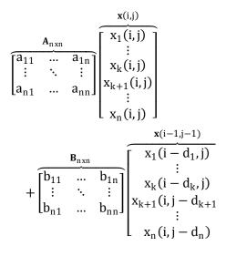
in which the over-braced  $\mathbf{x}(*, *)$ ,  $\mathbf{A}_{nxn}$  and  $\mathbf{B}_{nxn}$  are compact notations for the vectors and matrices, and the vectors in terms of x's represent the states of the system. Moreover, the matrices are all full ranked structures with real valued eigenvalues as well as real valued entries.
