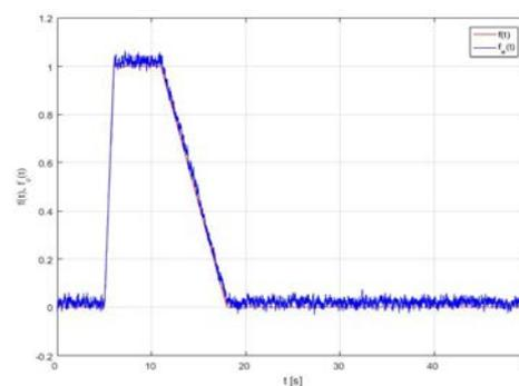
Fig. 2 Evolution of the first single actuator fault and its estimation with PD fault observer
