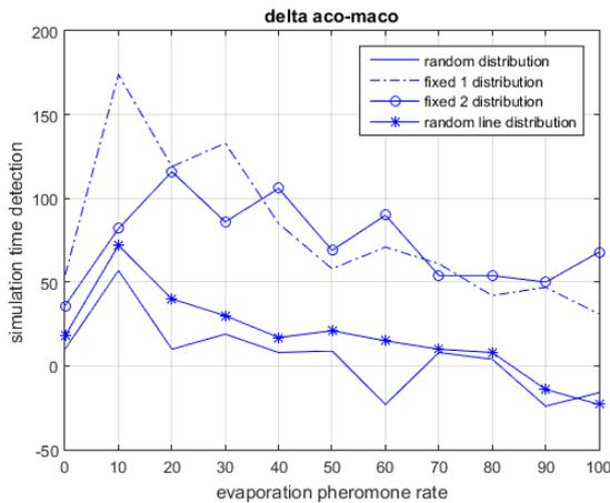
Fig. 10. Time detection comparison between ACO and modified ACO models
