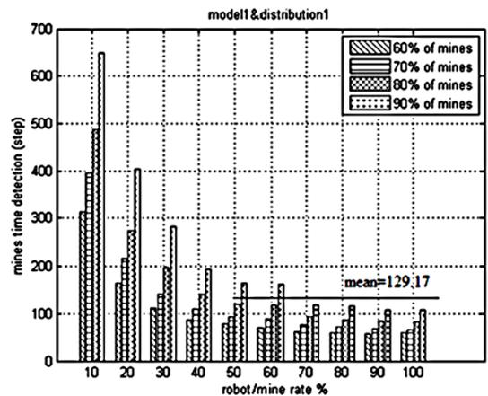
Figure. 7. Time detection mine using model BASE and random distribution.
