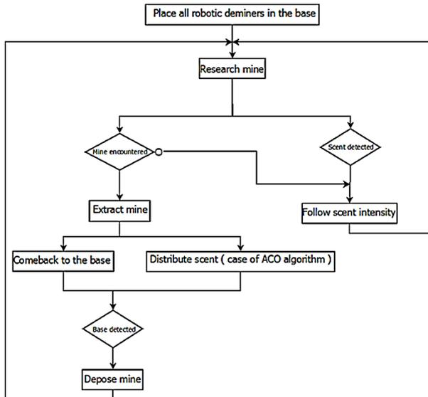
Fig. 5. Behavior diagram of a multi-robot demining system.
