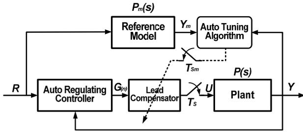
**Fig.1 Auto Regulation Control Configuration.**
