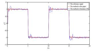
Fig.12 The output tracking curve of reference signal for  $y_2$
