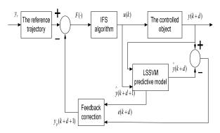
Fig.1 LSSVM predictive control model based on IFS algorithm **4.2 The algorithm stability analysis**
